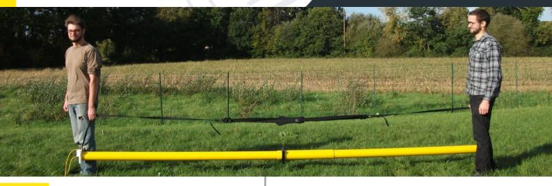
The DUALEM 421S has dual-geometry receivers at separations of 1, 2 and 3m from the transmitter, which provide four simultaneous depths of conductivity sounding, six simultaneous depths of susceptibility sounding, and detection of metal.
